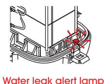
Water leak alert lamp
